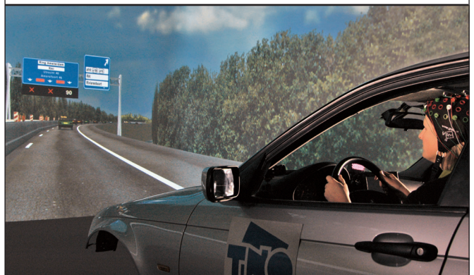
Figure 1. Using a BCI to assess driving performance. Brain signals might be useful in monitoring driver workload or evaluating in-vehicle systems that might interfere with the primary driving task.
