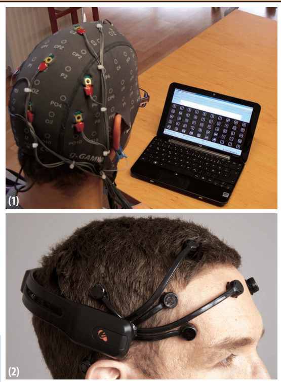
Figure A. Two BCI products in use. (1) The user is wearing electrodes while running IntendiX. (2) The user is wearing a band of dry EEG sensors developed by Emotiv.
